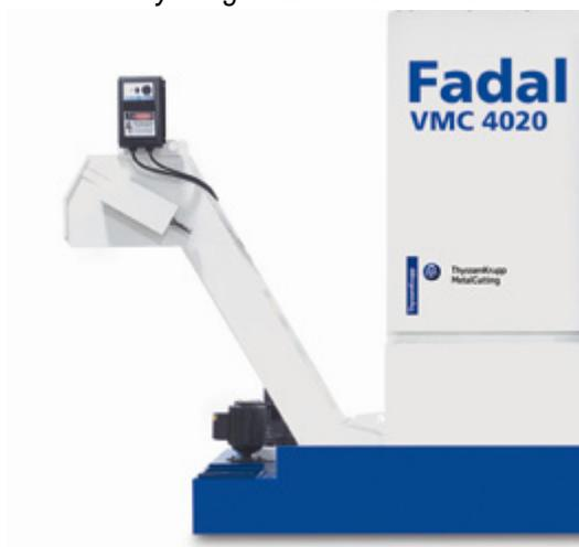
**Figure 3-15** Conveyor Against Left Side of Sheet Metal
