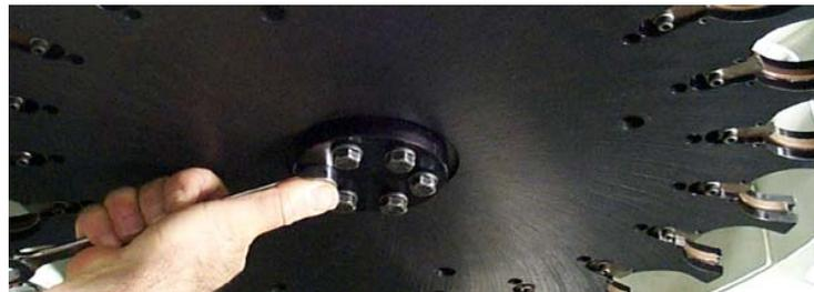
Figure 7-7: Loosen Hex Bolts Holding Tool Carrier
