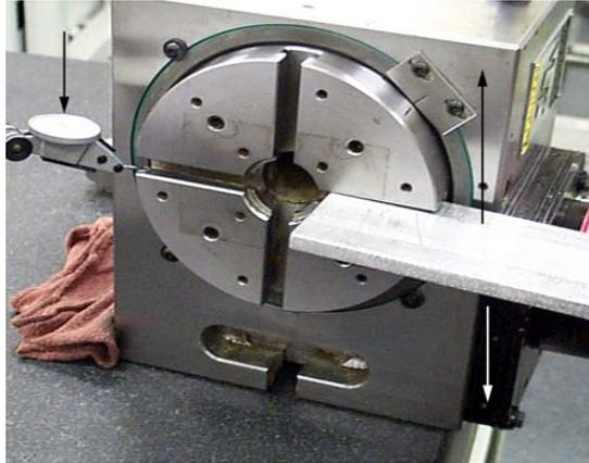
*Figure 8-12: Place Force on Plate*
