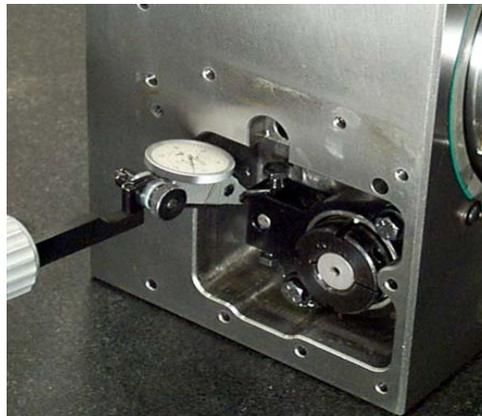
*Figure 8-7: Zero Indicator on Worm Pivot Plate*
