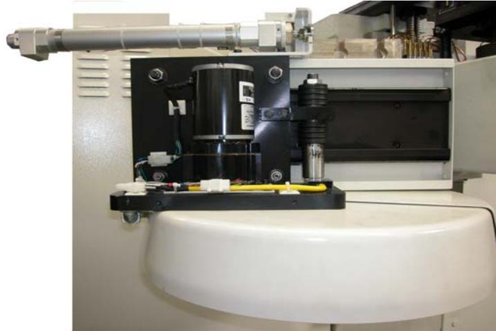
*Figure 7-2: Move ATC Slide Toward Spindle*
