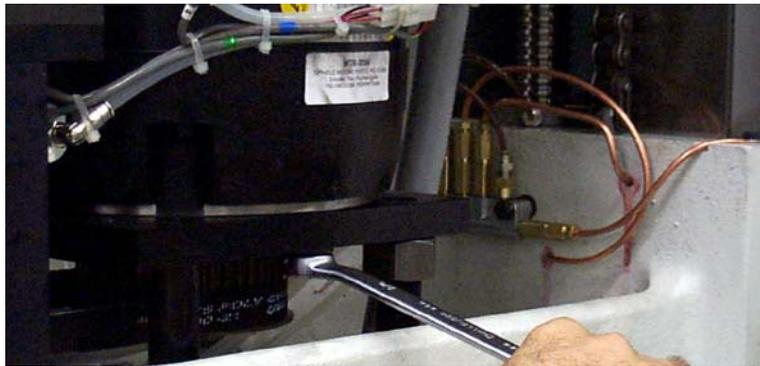
*Figure 10-14:* Loosen Hex Bolts to Spindle Motor
