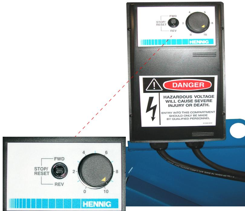
Figure 3-18: Control Operating Positions
