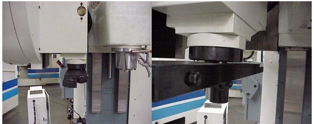
Figure 7-24: Place Taper Lock and Arm Assembly into Tool Changer Spindle
