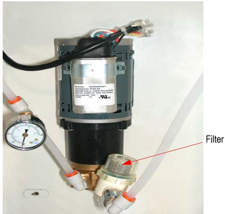
**Figure 4-1 Pump Filter**
