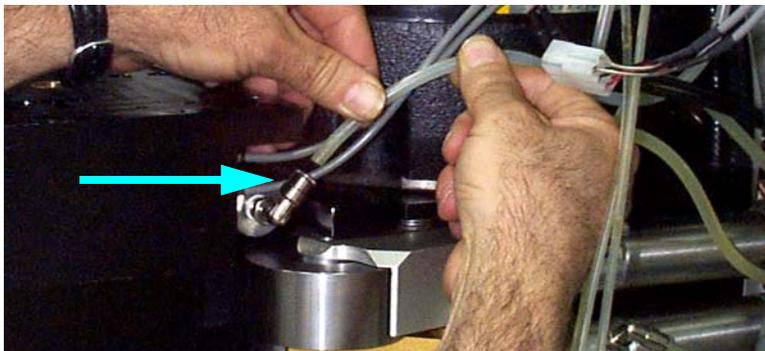
*Figure 10-4: Disconnect Air Line to Orientation Piston*
