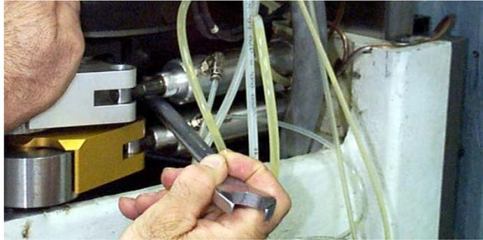
*Figure 10-8:* Remove Spindle Motor Bolt
