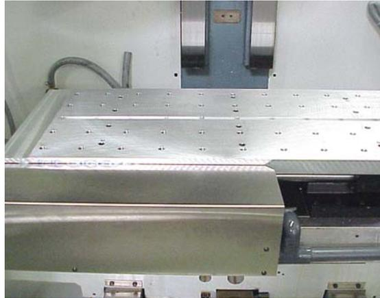
*Figure 9-3 Remove Pallet Arm Safety Cover*
